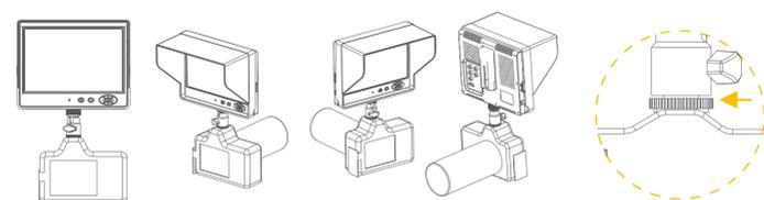
After attaching the shoe adapter to the monitor, mount the shoe adapter to the camera hot shoe, then lock the shoe adapter by rotating the shoe adapter locking screw C.
