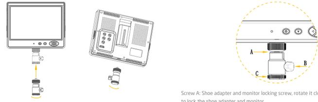
Attach the shoe adapter to the 1/4" screw hole at the bottom of the monitor and lock it by rotating the adapter clockwise.
