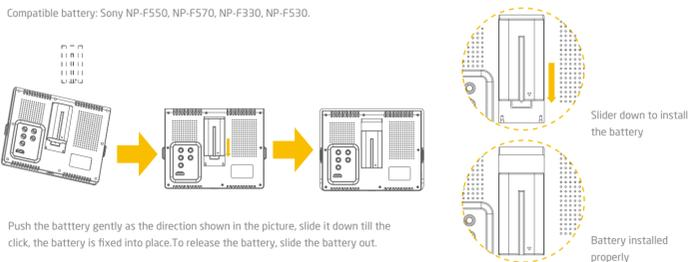
Push the battery gently as the direction shown in the picture, slide it down till the click, the battery is fixed into place. To release the battery, slide the battery out.
