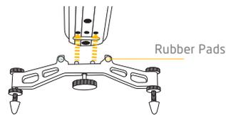
2. Tighten the thumb screw until tight and the leg is secure.
