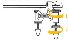
8. Tighten the locking nuts by tightening them against the frame of the leg.
