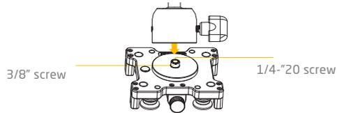
Note: the mounting screw may need to be tightened with an Allen key (not included).
