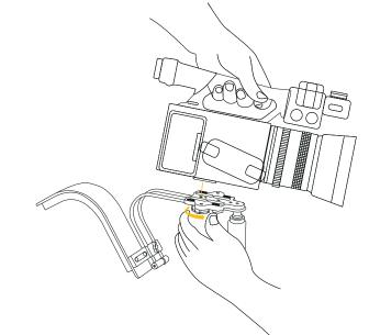
7. Adjust the distance of the camera from your eye by loosening the baeplate mounting screw slightly and sliding the camera forward or back to the desired position. Tighten the screw securely. Do not overtighten.
