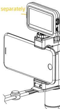
6. Remove the hand grip, SK-PSC1 can be mounted onto the tripod with the built in 1/4" screw at the bottom of the phone holder.
