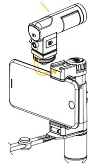
2. Mount SK-PSC1 to a tripod with the built in 1/4 screw thread at the bottom of the hand grip.
